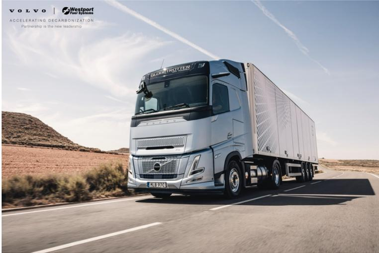
*Caption: The Volvo FH Aero gas-powered was launched IN 2024. It brings performance and productivity like a diesel-powered truck and sufficient range for long-haul transport. The HPDI™-equipped Volvo FH truck can reduce CO<sub>2</sub> emissions by up to 100 percent. This is calculated from tank to wheel when using bio-LNG and HVO, compared to a truck using European standard diesel.*
