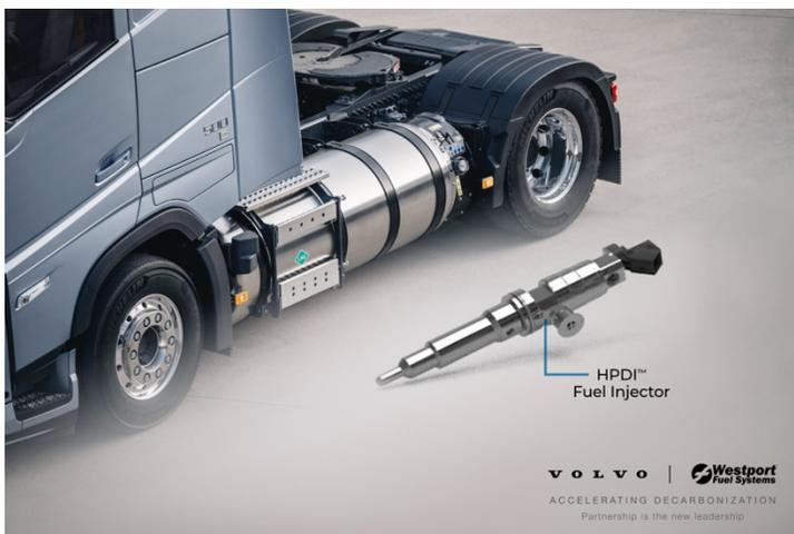
*Caption: At the heart of the HPDI™ Fuel System is a revolutionary patented injector with a dual concentric needle design that delivers small quantities of diesel fuel and large quantities of natural gas, at high pressure, to the combustion chamber. The natural gas is injected at the end of the compression stroke. Launched in 2024, the Volvo FH Aero gas-powered is a long-haul truck shaped for aerodynamic efficiency.*
